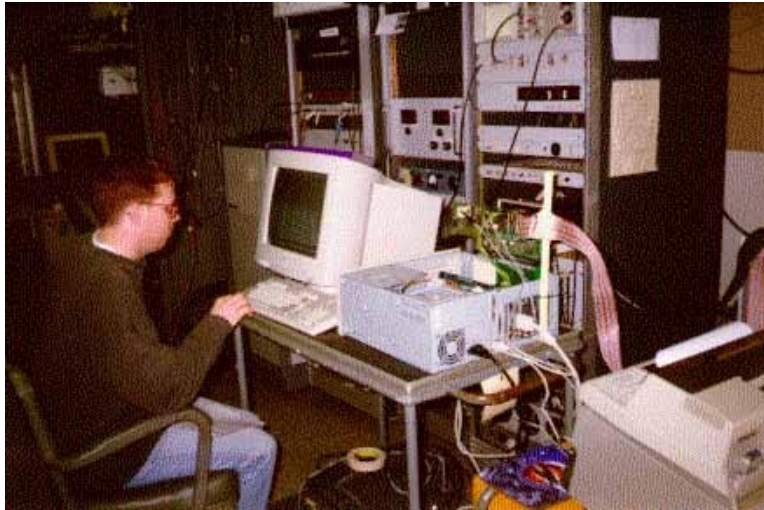
Figure 5-5: A photograph of the NRTC installed in the control room of the GB140' telescope. The two ribbon cables on the right carry the data being correlated.
